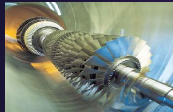
Gas Turbine Rotor
