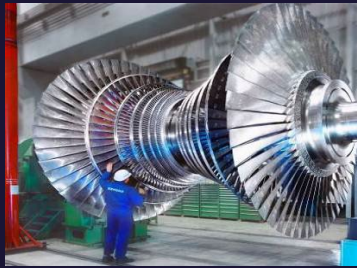
Steam Turbine LP
